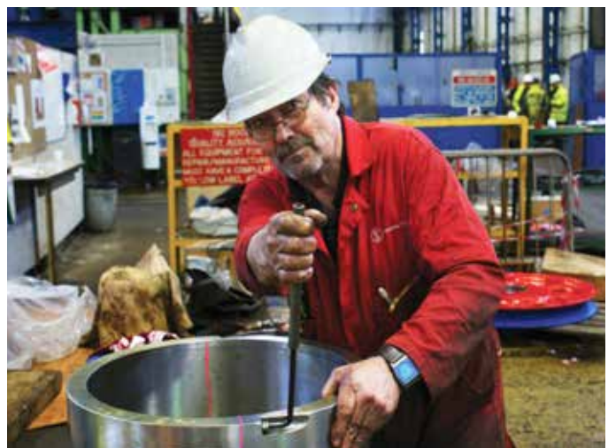
an engineer at work on a sterntube liner
