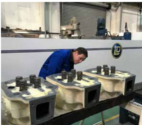
reconditioning of components
